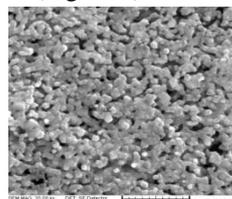
Figure 2. - SEM micrograph of (BTL) ceramics of a sintered sample
