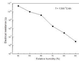
Figure 3. - Electrical resistance vs. relative humidity for BTL
