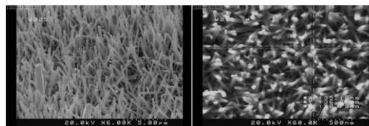
Fig. 1 – SEM images showing the synthesized ZnO nanowires. The average nanowire diameter is 50nm.
