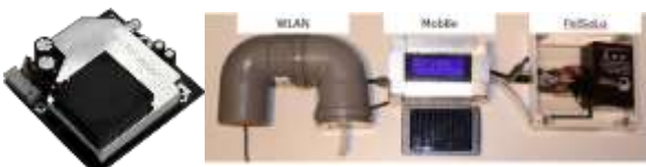
Fig 1: left: SDS011-sensor;right: developed PM-modules
