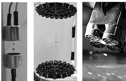
Figure 1–3 – Small levitator, big levitator, ultrasonic stick (from left to right)
