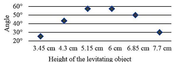
Figure 4 – The tilt of the levitator when the levitating object falls
