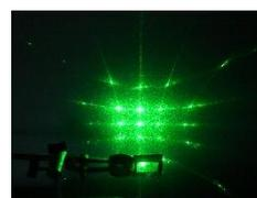
Image 3 - Diffraction pattern created by shining a laser through two perpendicular gratings
