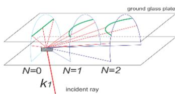
Image 2- Diffraction by linear grating shown on ground glass plate in physical space
