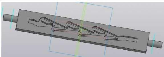
Fig.1 3D model of the Tesla valve
