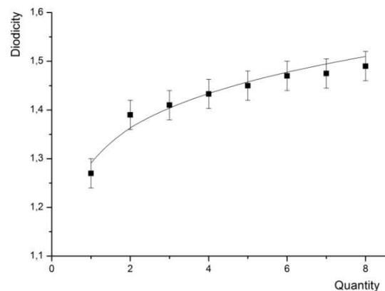
Graph 1 – The dependence of the Diodicity by the quantity of stages.
