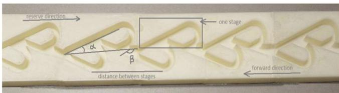
Fig.2 printed Tesla valve
