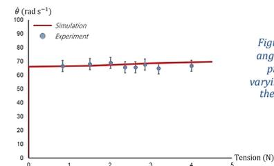
Figure 4: Graph of angular velocity of propeller with varying tension along the tied diagonal.
