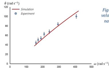
Figure 3: Graph of angular velocity of propeller against natural frequency of rod.
