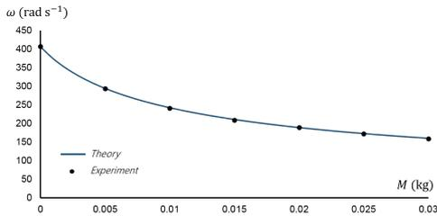
Figure 1: Calibration graph of experimentally and theoretically-determined  $\omega$  with varying  $M$ .
