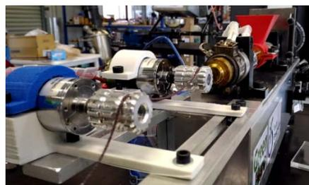
Figure 3: Overall extrusion process using GreenHero Mini-Extruder
