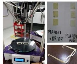
Figure 6: PLA/NR blends products fabricated by a Fused-Deposition Modeling 3D printer.
