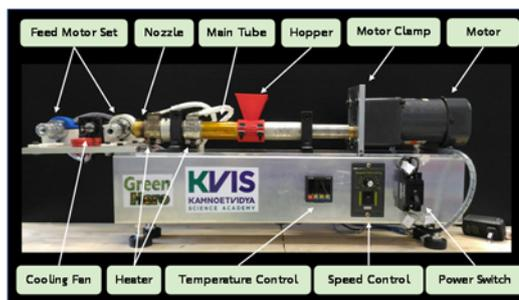
Figure 2: Components of GreenHero Mini-Extruder (Size: 20x79x30 cm, Weight: 11.5 Kg)
