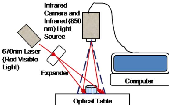
Figure 1. Measurement System
