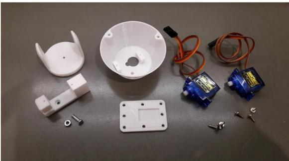
**Figure 1.** Printed parts and servo motors
