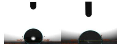
Figure 3.3. Bio-TPU and K-TPU contact angle
