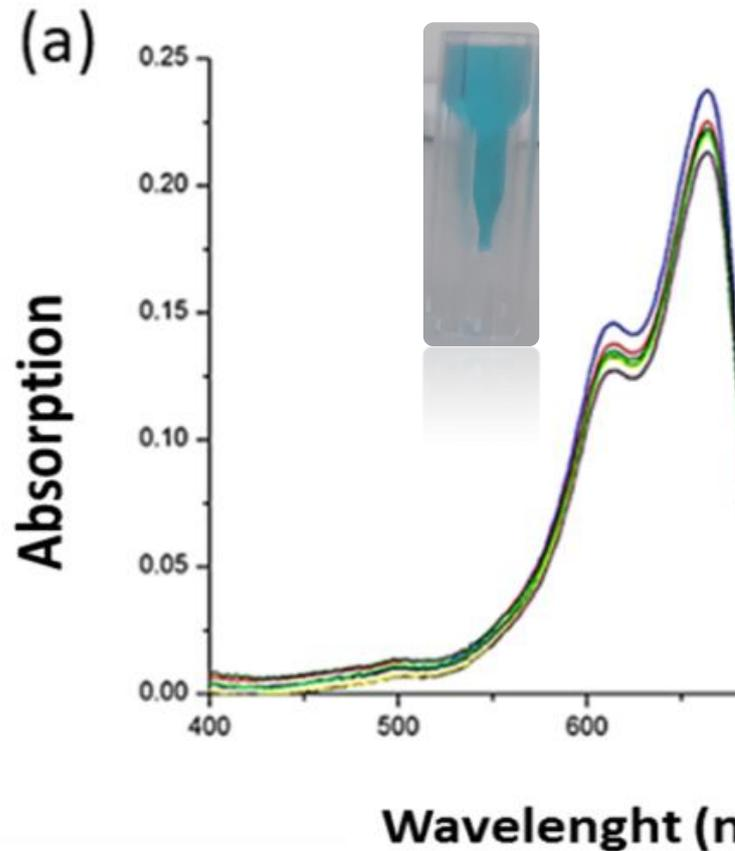
Figure 3. a) The control group (b) The absorption measurement of the TiO<sub>2</sub>-coated glass bowl with the spectrophotometer
