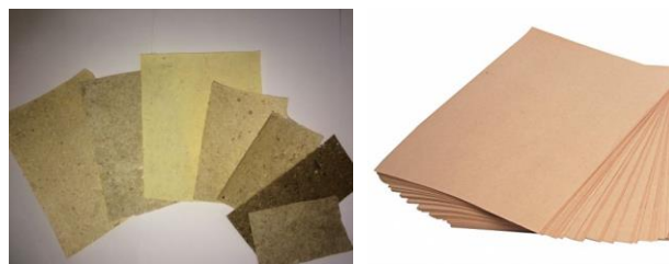
Fig.4. The result of paper making/ The density in this photo is 70 g/m 2
